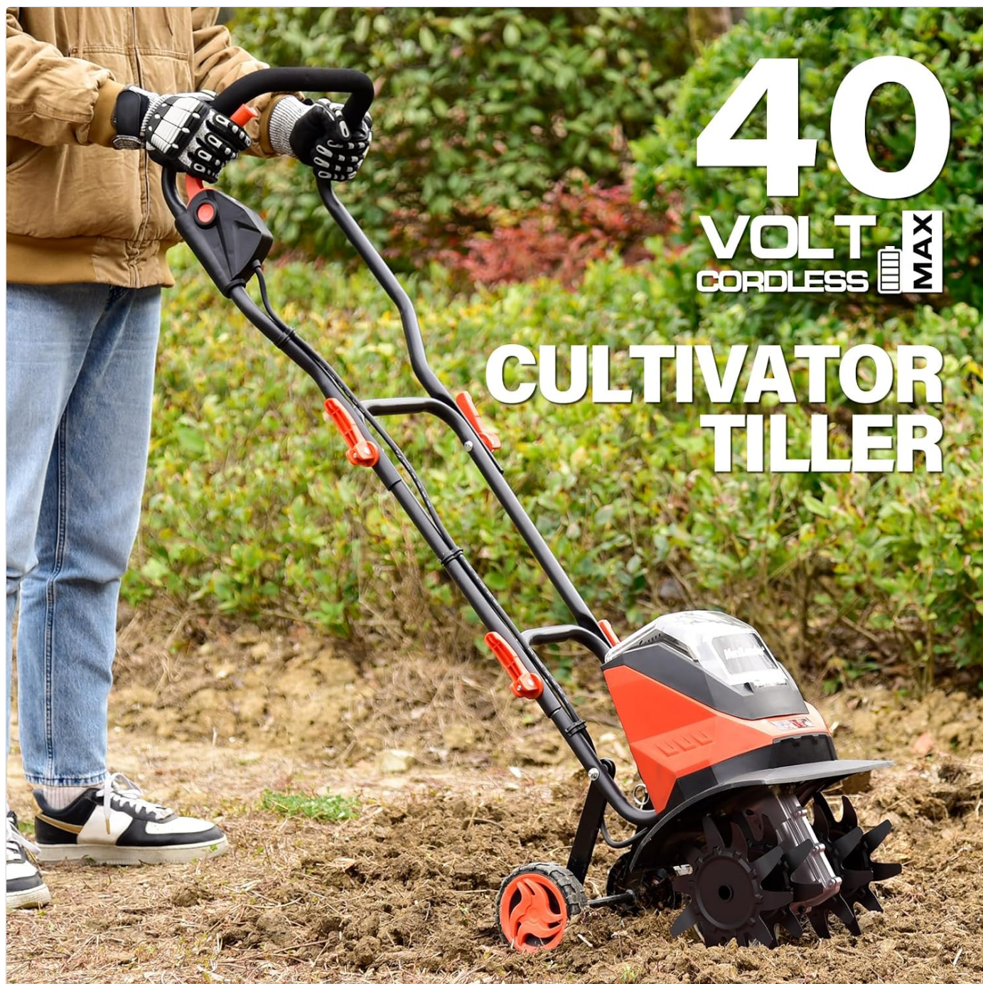
Figure 4.2: Tiller in operation. The tines rotate to break up and aerate the soil.
