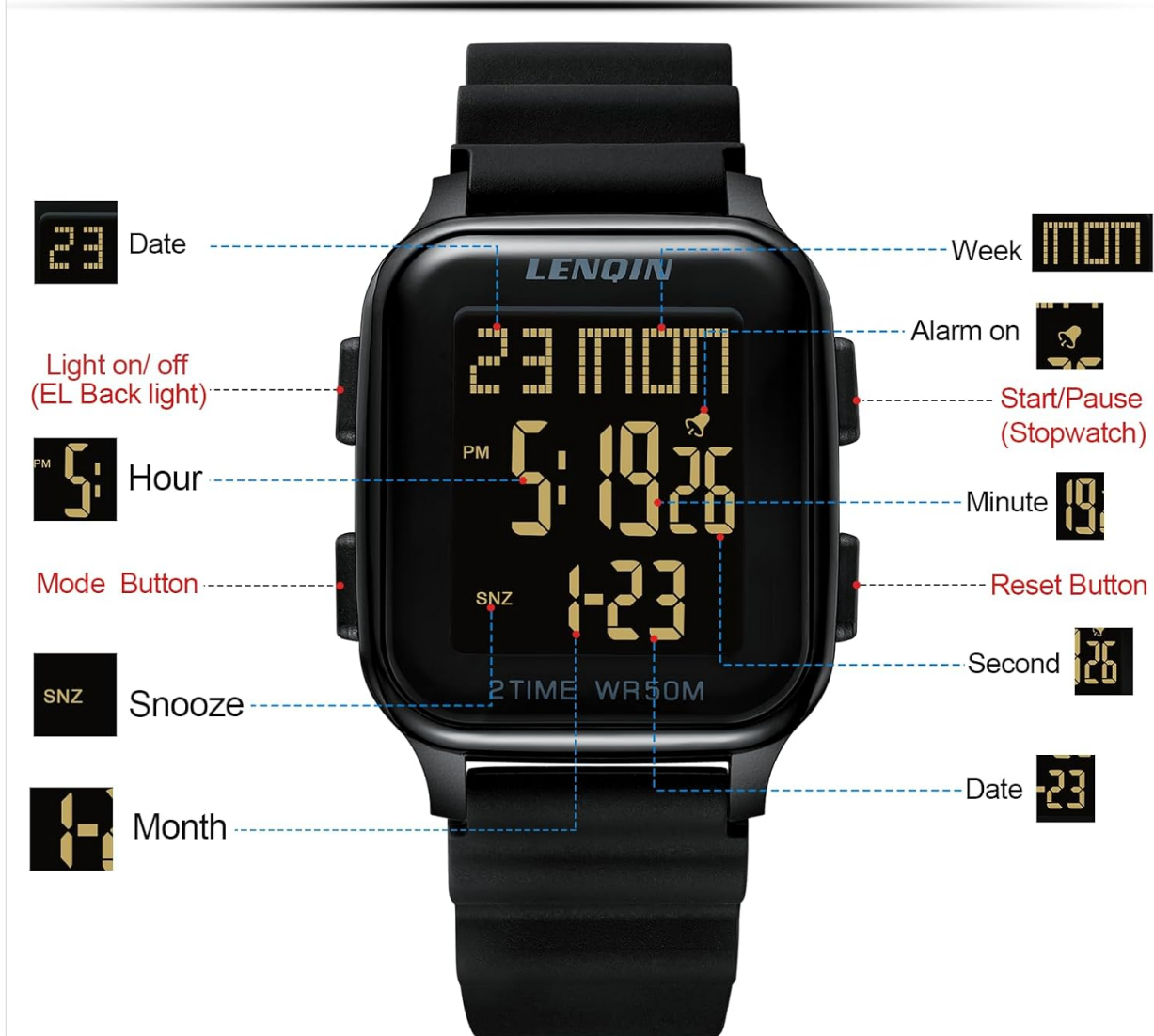
Image 3.1: Diagram illustrating the LN LENQIN R027 watch's display elements and button assignments. The display shows Date, Week, Alarm on indicator, Hour, PM indicator, Minute, SNZ (Snooze) indicator, Month, and Date. Buttons are labeled for Light on/off (EL Backlight), Mode Button, Start/Pause (Stopwatch), and Reset Button.
