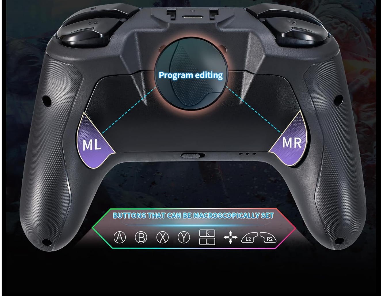
Figure 4.2: Macro Programming Interface. This image highlights the "Program editing" area on the back of the controller, indicating the ML and MR buttons and the range of buttons that can be mapped (A, B, X, Y, R, L, ZL, ZR, D-pad directions).
