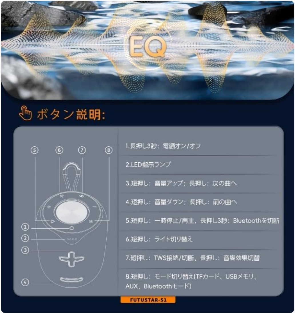
Image: Diagram illustrating the speaker's control buttons and their functions.
