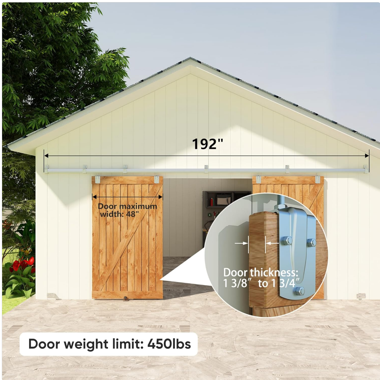
Image 4.1: This diagram illustrates the maximum door width of 48 inches, a compatible door thickness range of 1 3/8 to 1 3/4 inches, and a door weight limit of 450 lbs for the JUBEST barn door hardware kit.
