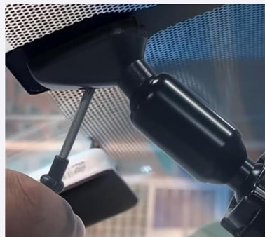
4. Tighten the screw on this bracket to fix it on the base.
