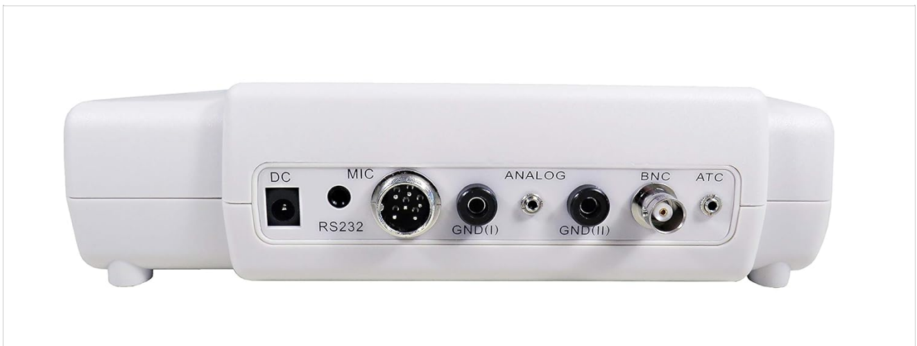
Figure 2.3: Rear panel connections of the Sper Scientific 860031. From left to right: DC power input, RS232 port, Analog output (GND and Signal), BNC connector for pH electrode, and ATC probe input.
