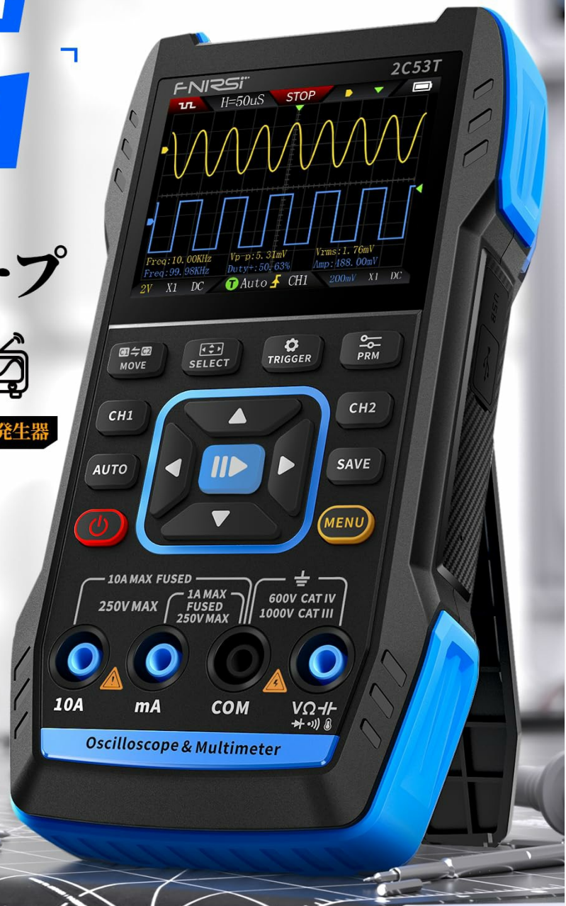
Figure 2.1: Front view of the FNIRSI 2C53T, showing the display, control buttons, and input terminals.
