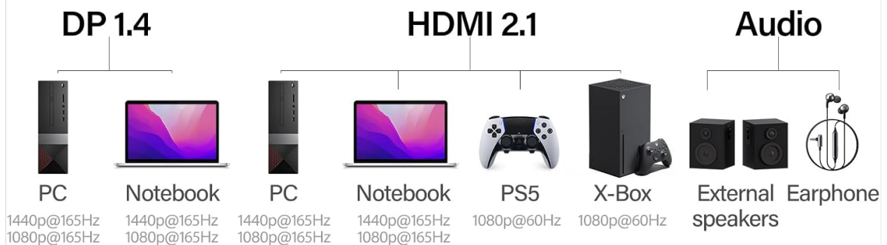
Figure 4: Visual guide for GPU compatibility and recommended port types (DP 1.4, HDMI 2.0 or later) for optimal display performance.
