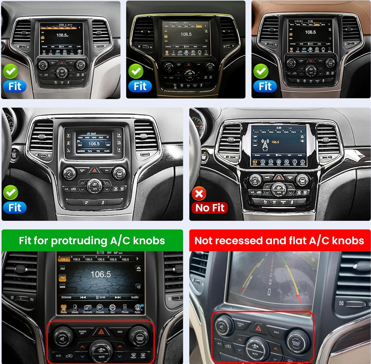
Figure 3.1: Compatible and Incompatible Dashboards. Ensure your vehicle has protruding A/C knobs for proper fitment. Models with recessed and flat A/C knobs are not compatible.
