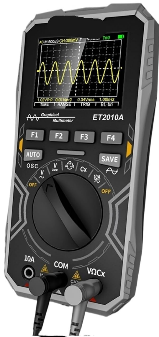
Figure 3.1: Front view of the TOOLTOP ET2010A. This image shows the device from a front-right angle. The screen displays an oscilloscope waveform. Probes are connected to the 10A and VΩCx input jacks. The rotary dial is set to an oscilloscope function.
