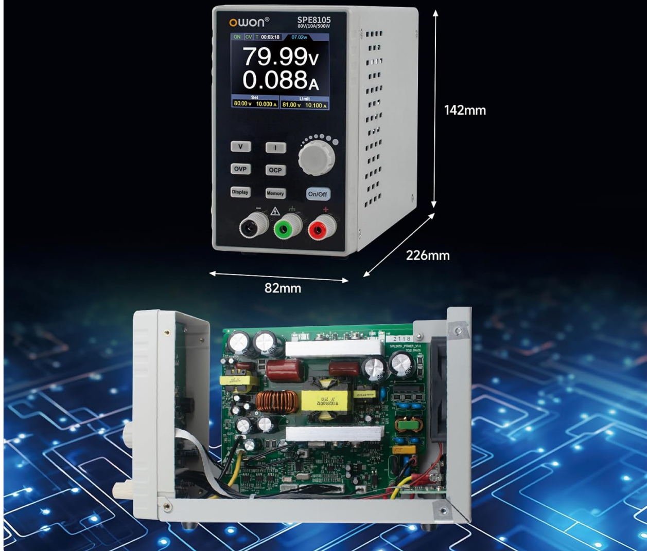
Figure 5: OWON SPE8105 dimensions and internal component layout.
