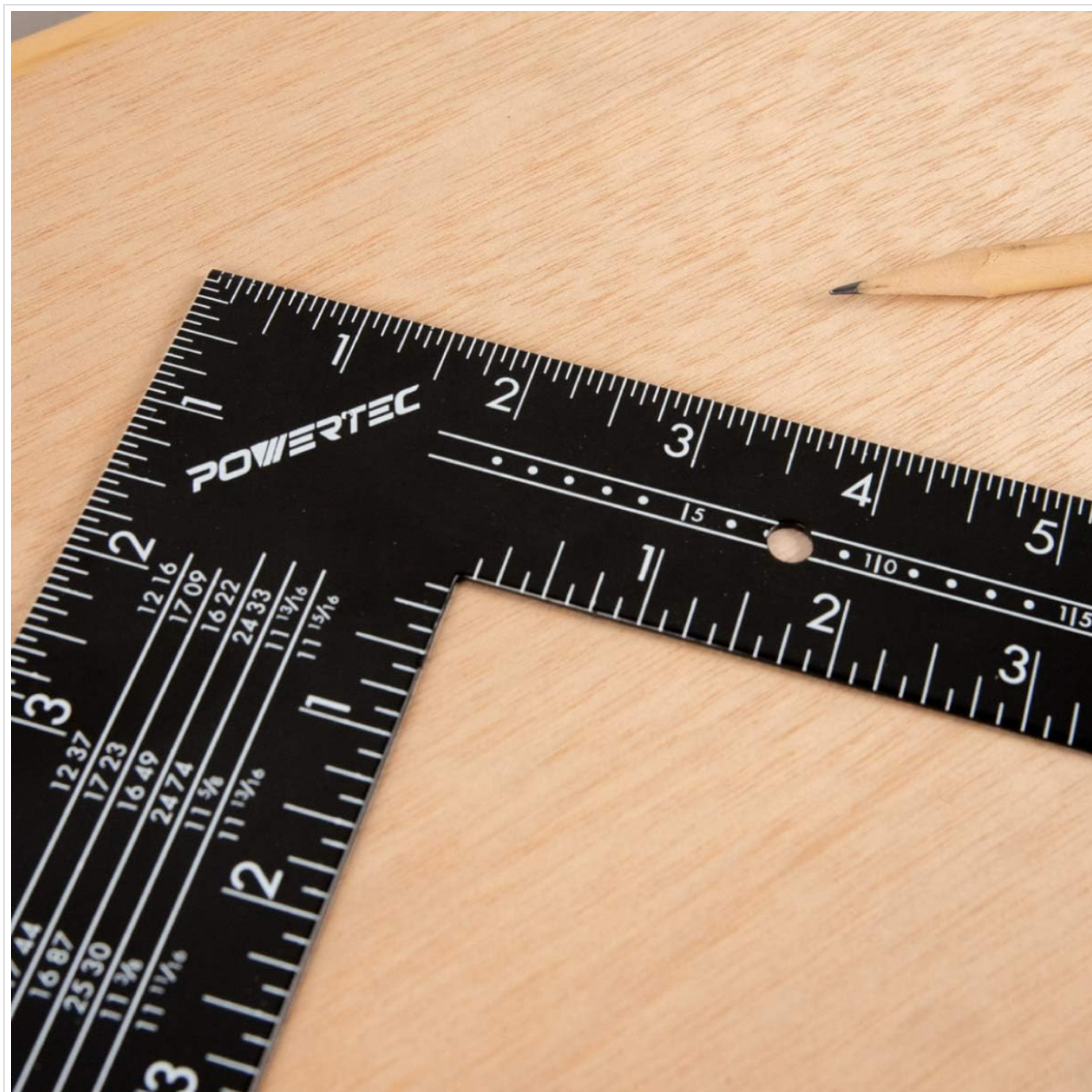
Image 4.2: Detailed view of the rafter tables etched onto the framing square, providing quick reference for roof framing calculations.
