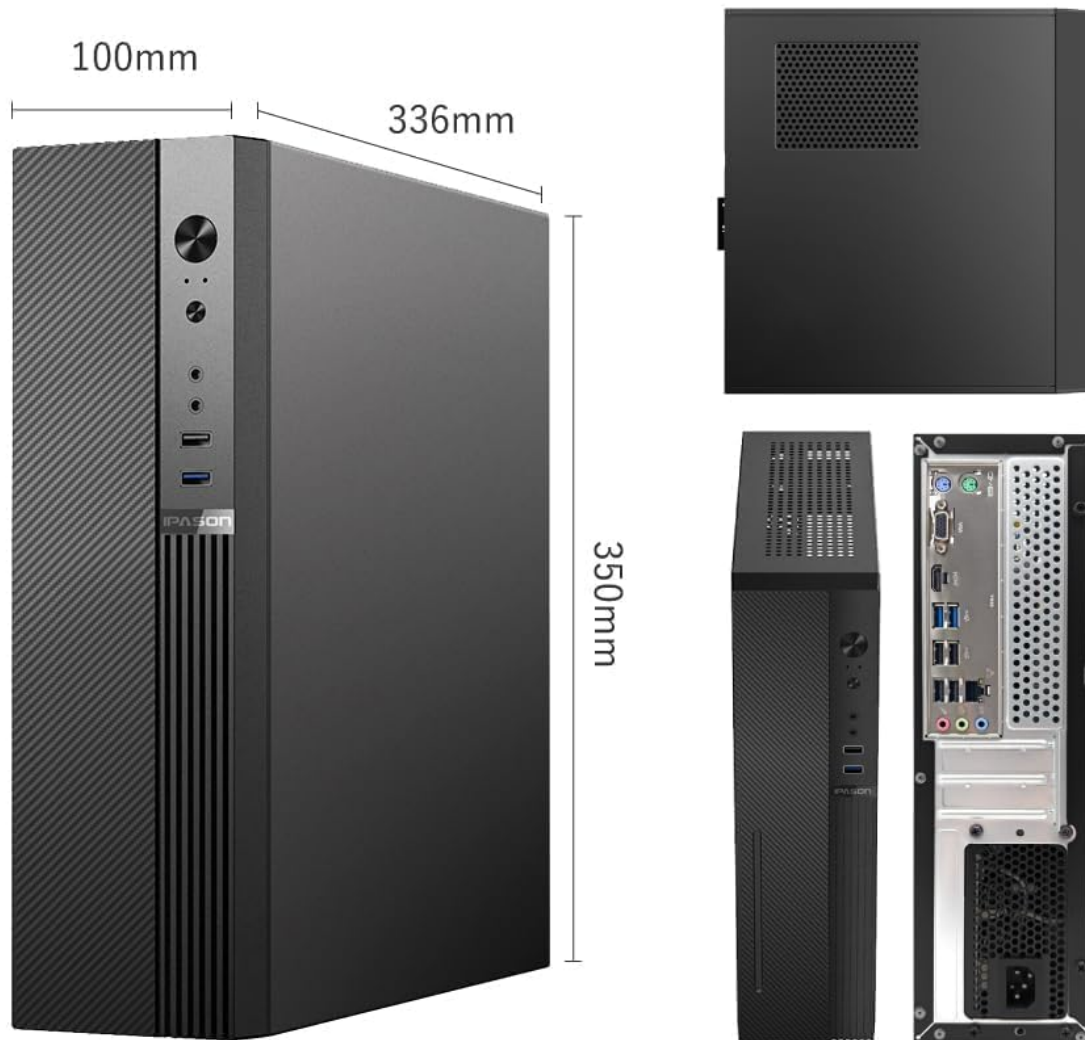
Figure 2: Detailed dimensions of the IPASON G-SLIM Desktop PC, illustrating its compact form factor (100mm width x 336mm depth x 350mm height).
