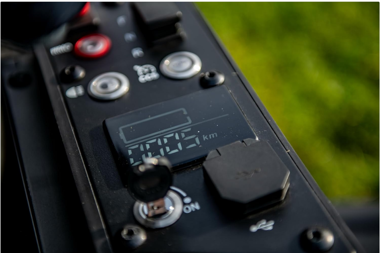
Figure 3: The integrated LCD display provides real-time battery status and mileage tracking.
