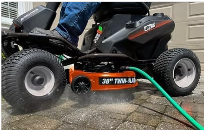
Figure 7: The cutting deck can be easily cleaned by attaching a hose to the wash port and running the blades briefly (refer to manual for detailed steps).
