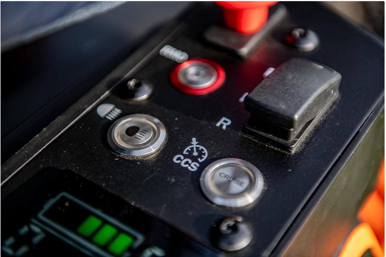
Figure 4: The control panel features a drive selector (F-N-R for Forward, Neutral, Reverse) and a cruise control button (CCS).
