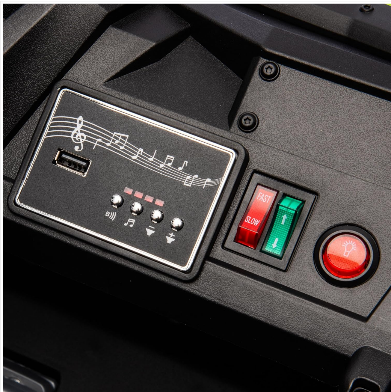
Image: The control panel of the UTV, showing buttons for music, horn, and speed selection (Fast/Slow).
