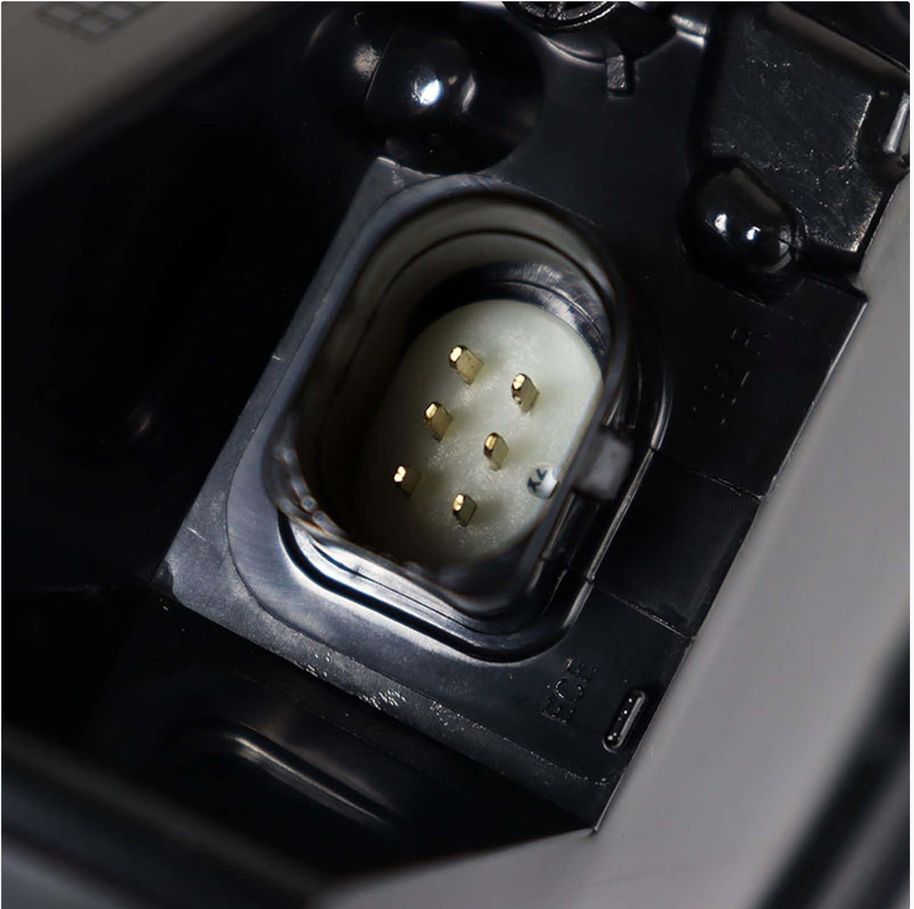
Figure 3: Electrical connector detail. This image shows the multi-pin electrical connector for the tail light, indicating its plug-and-play design.
