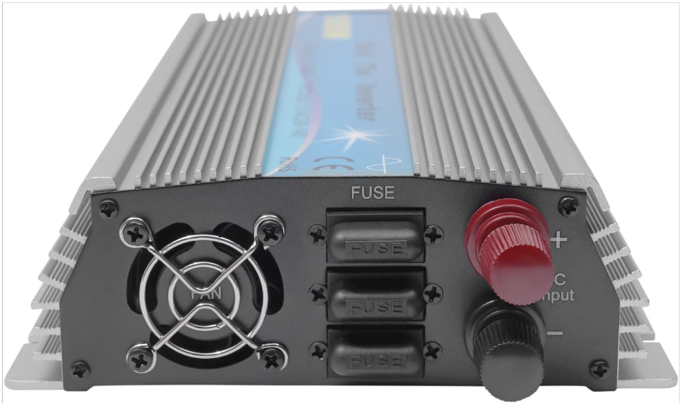
Figure 2: Rear view showing DC input terminals, cooling fan, and fuse access points.
