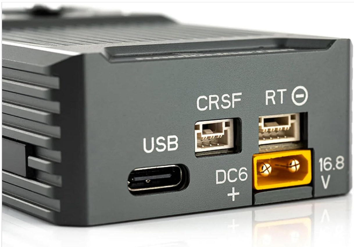
Figure 4.3: Side view showing the various connection ports: USB-C, CRSF, RT, and the XT30 power input (DC 6V-16.8V).
