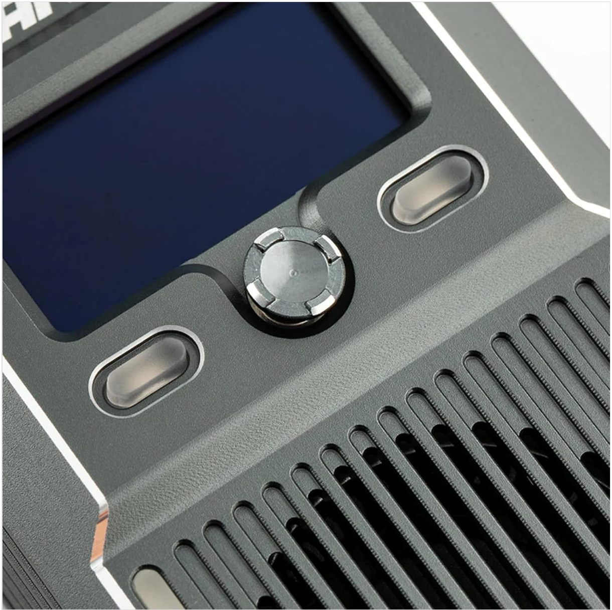
Figure 4.2: Detailed view of the module's user interface, including the high-contrast OLED display and the 5-directional navigation key for menu interaction.
