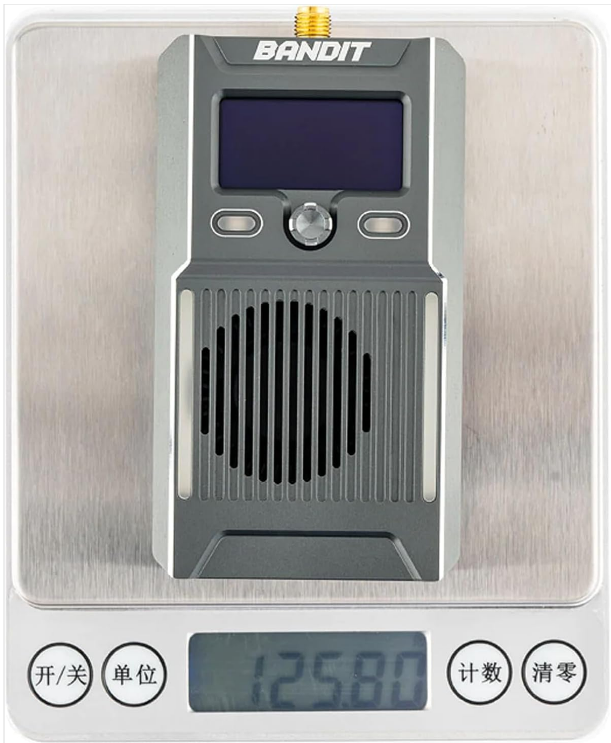
Figure 9.1: The Bandit RF Module on a scale, indicating its weight for reference.
