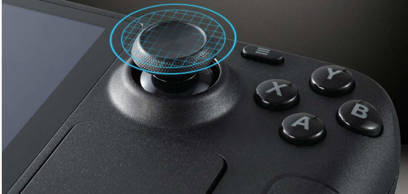
Image: Close-up of a joystick cap highlighting its touch-sensing functionality.
