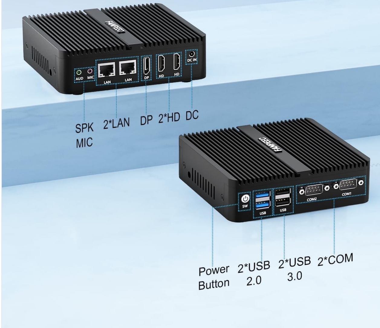
Figure 3.3: Front and Rear Port Layout.
