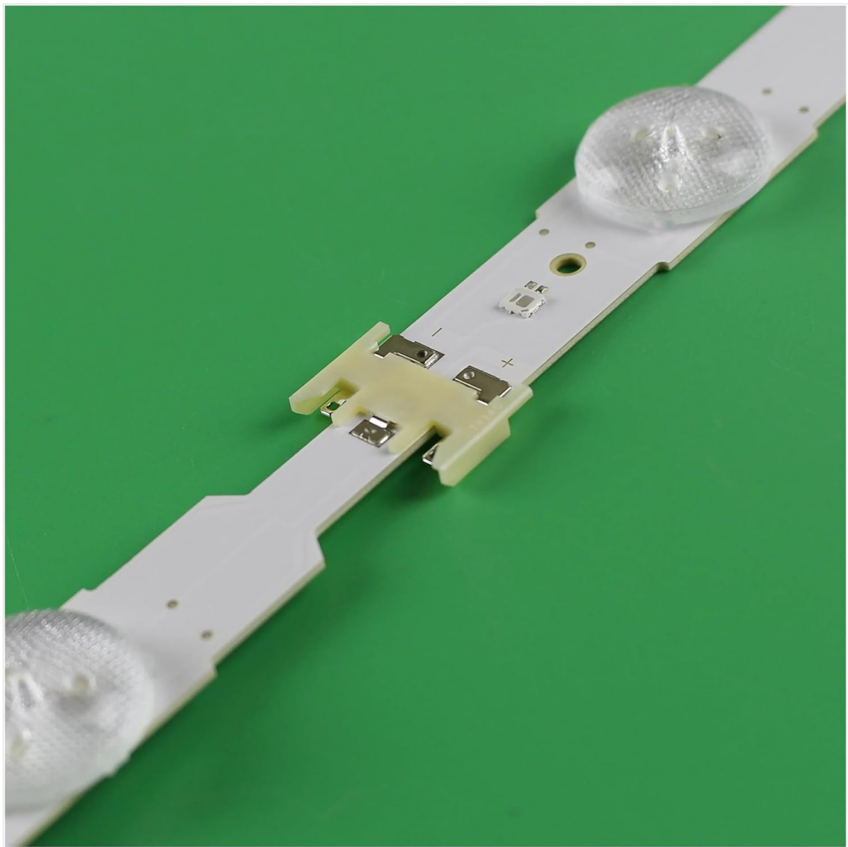
Image: Detailed close-up of the electrical connector on an LED backlight strip, showing the pins and housing.
