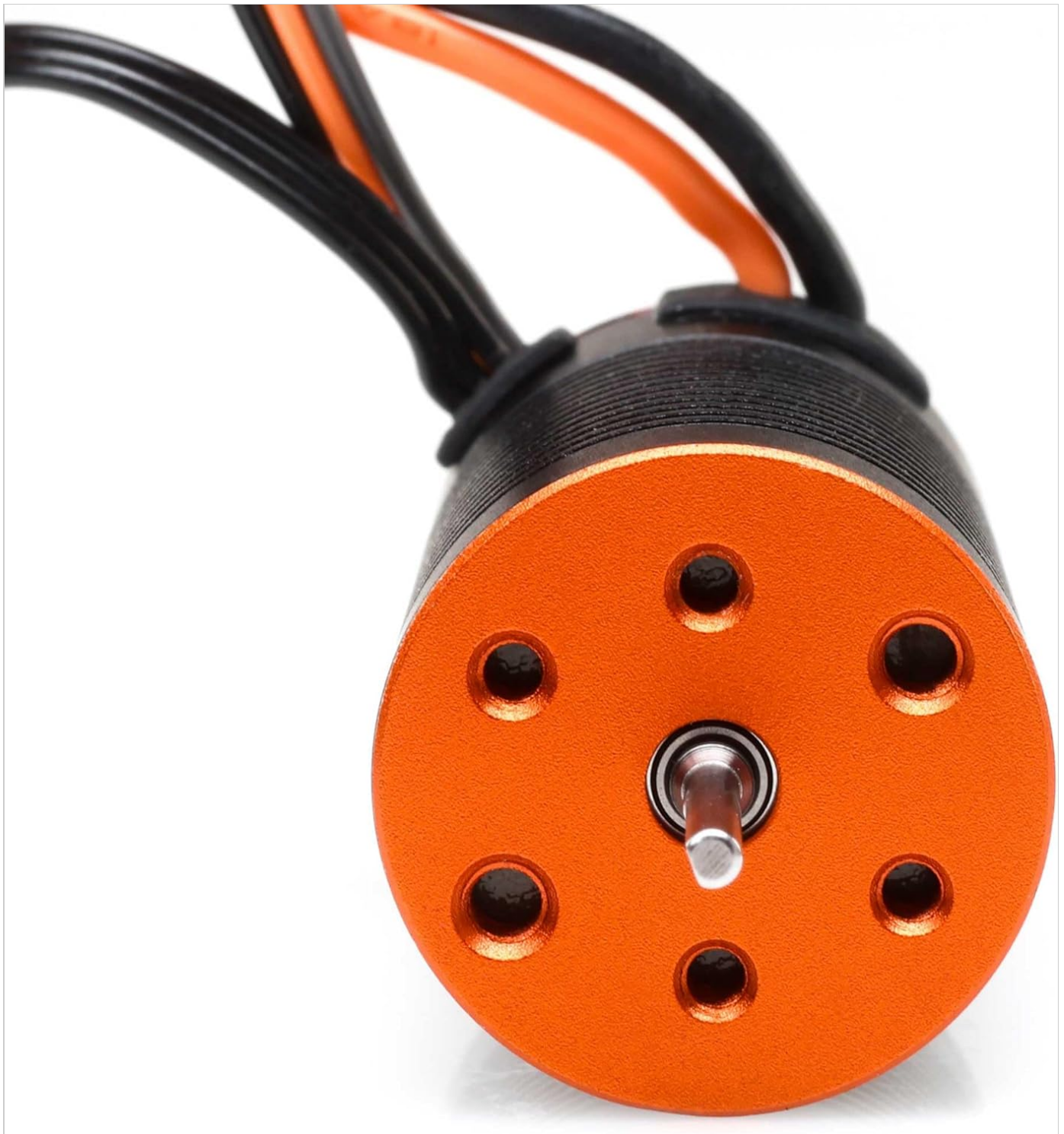
Figure 3: Close-up view of the motor/ESC combo showing the integrated wiring for connection to the receiver and battery.
