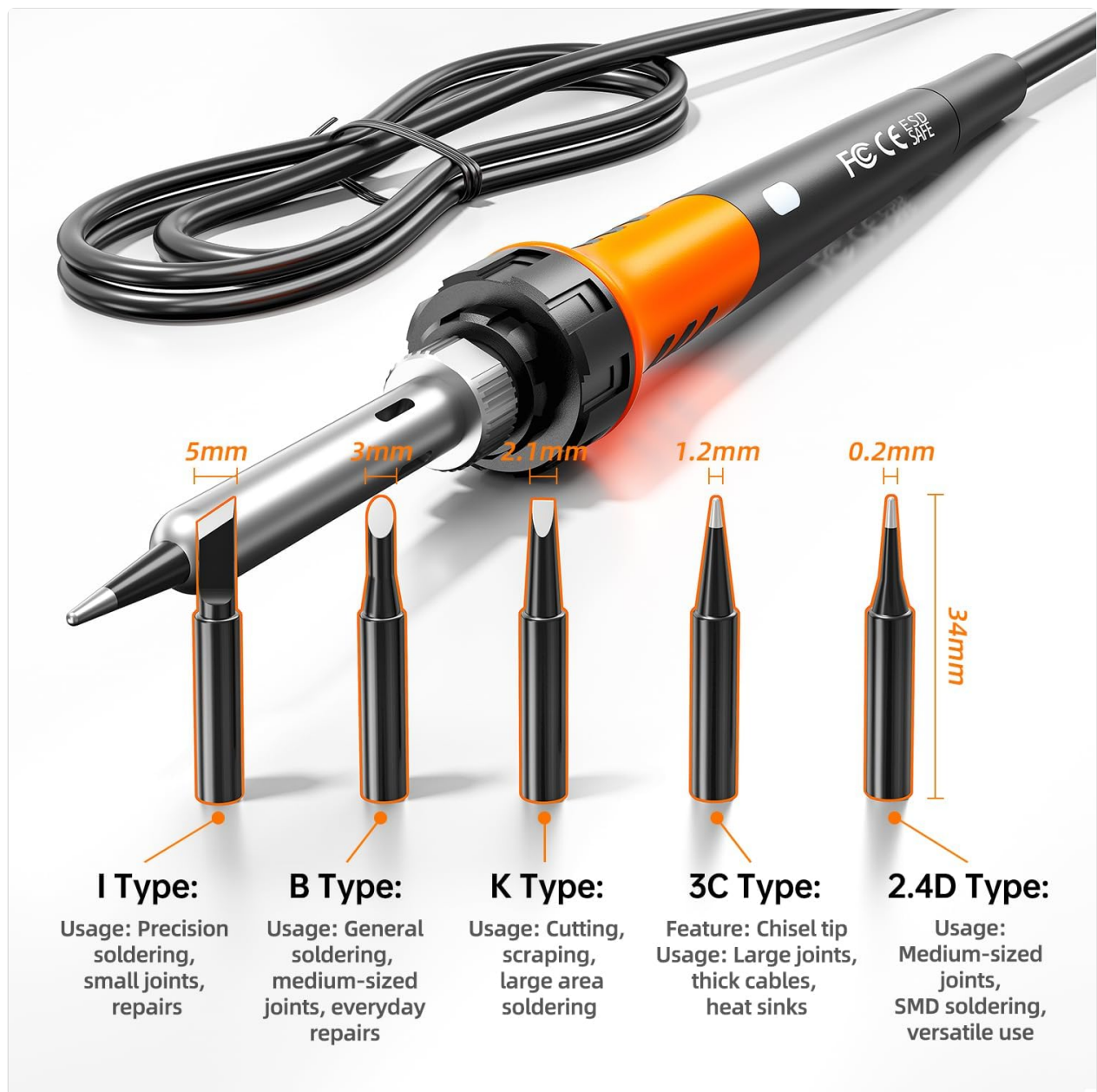
Figure 3: Various soldering tip types (I, B, K, 3C, 2.4D) with their dimensions and recommended usage, such as precision work, general soldering, cutting, and large joints.
