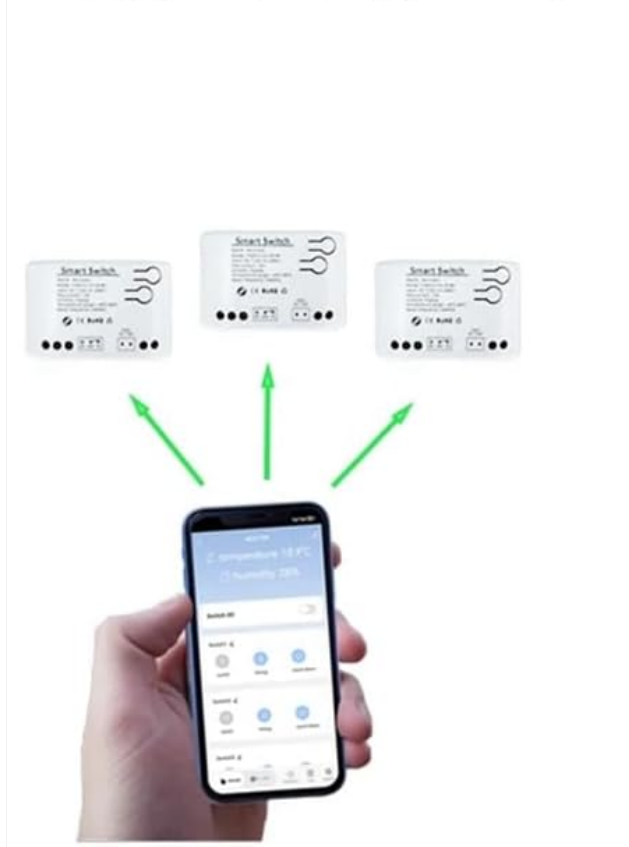
Image 4: Illustration showing how one person can control multiple smart switches, and how multiple people can share control over a single smart switch using a mobile application.
