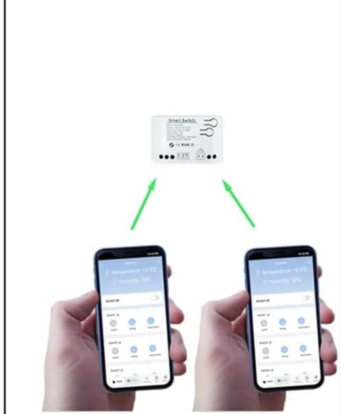
Image 4: Illustration showing how one person can control multiple smart switches, and how multiple people can share control over a single smart switch using a mobile application.
