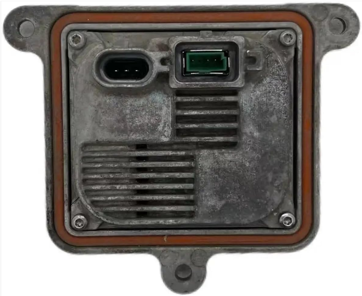
Figure 4.2: Rear view of the ballast unit, illustrating the main power input connector and the output connector for the D3S bulb, along with integrated heat dissipation fins.
