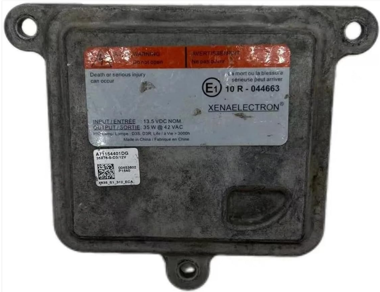
Figure 4.1: Front view of the LBAXXP Xenon D3S Headlight Ballast Unit. The label clearly displays the model number 10R-044663, input voltage of 13.5V DC, and output of 35W at 42V AC, along with safety warnings.
