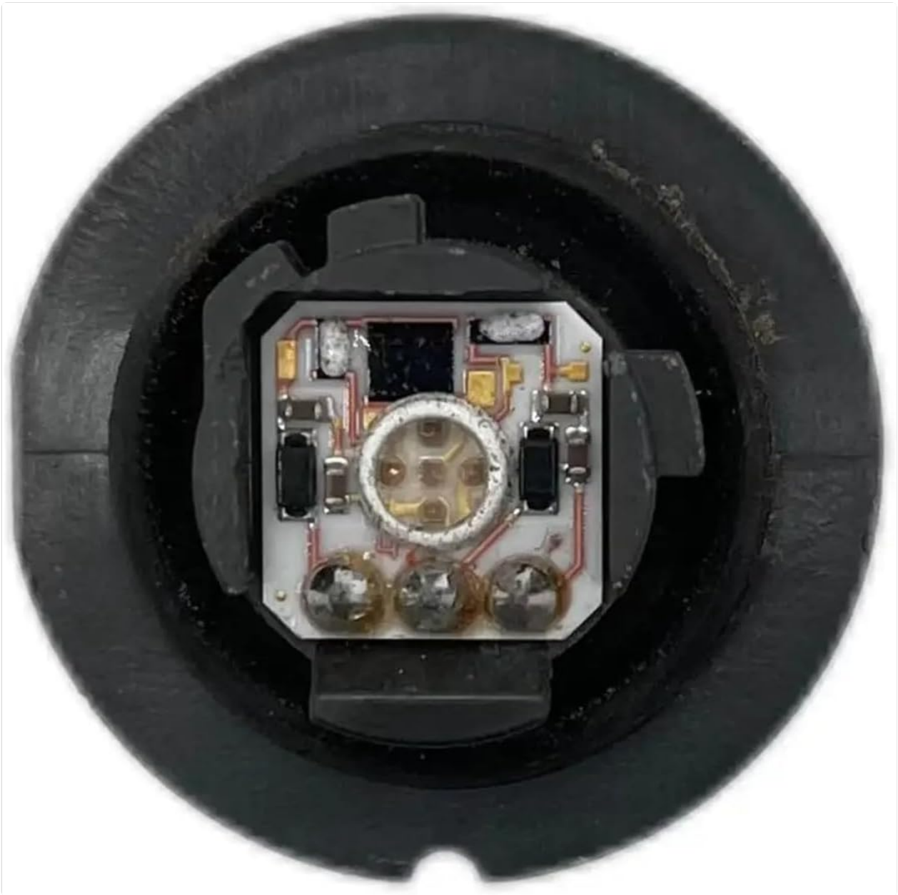
Image 1: Front view of the LED module, highlighting the light-emitting diodes and internal circuitry.
