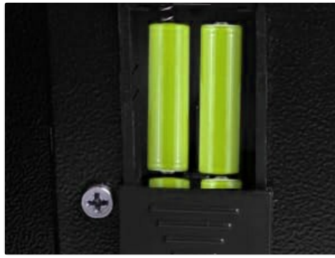
Image 5.1: Battery compartment for the electronic keypad.
