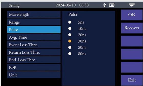
Figure 5: Screenshots illustrating the Automatic OTDR and Expert OTDR modes with parameter settings.
