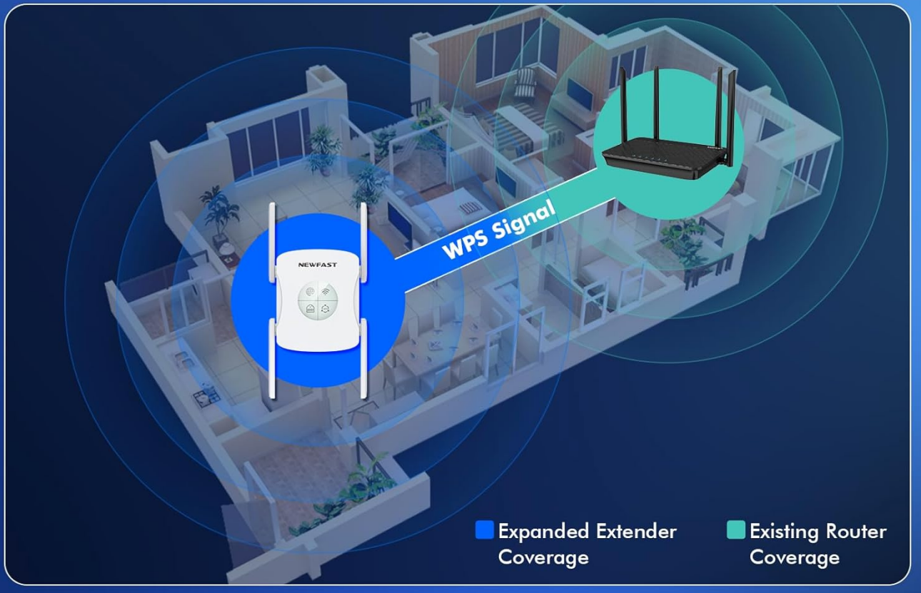
Image 3.1: Illustration of the WPS one-key connection process between a router and the NEWFAST AX1800 extender.
