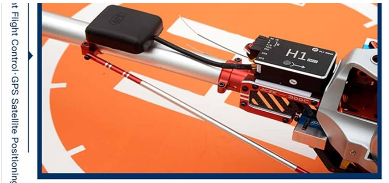
Figure 4.1: The H1 Smart Flight Controller enables precise GPS satellite positioning and enhanced stability.
