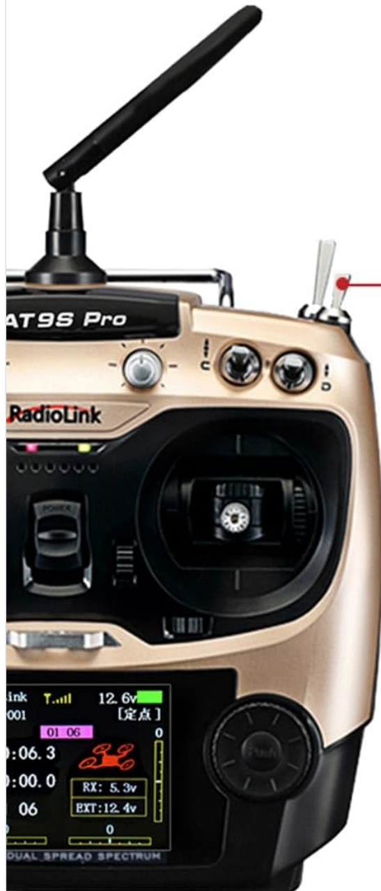
Figure 3.2: The AT9S PRO 12-channel remote control with LCD display, used for controlling the helicopter.
