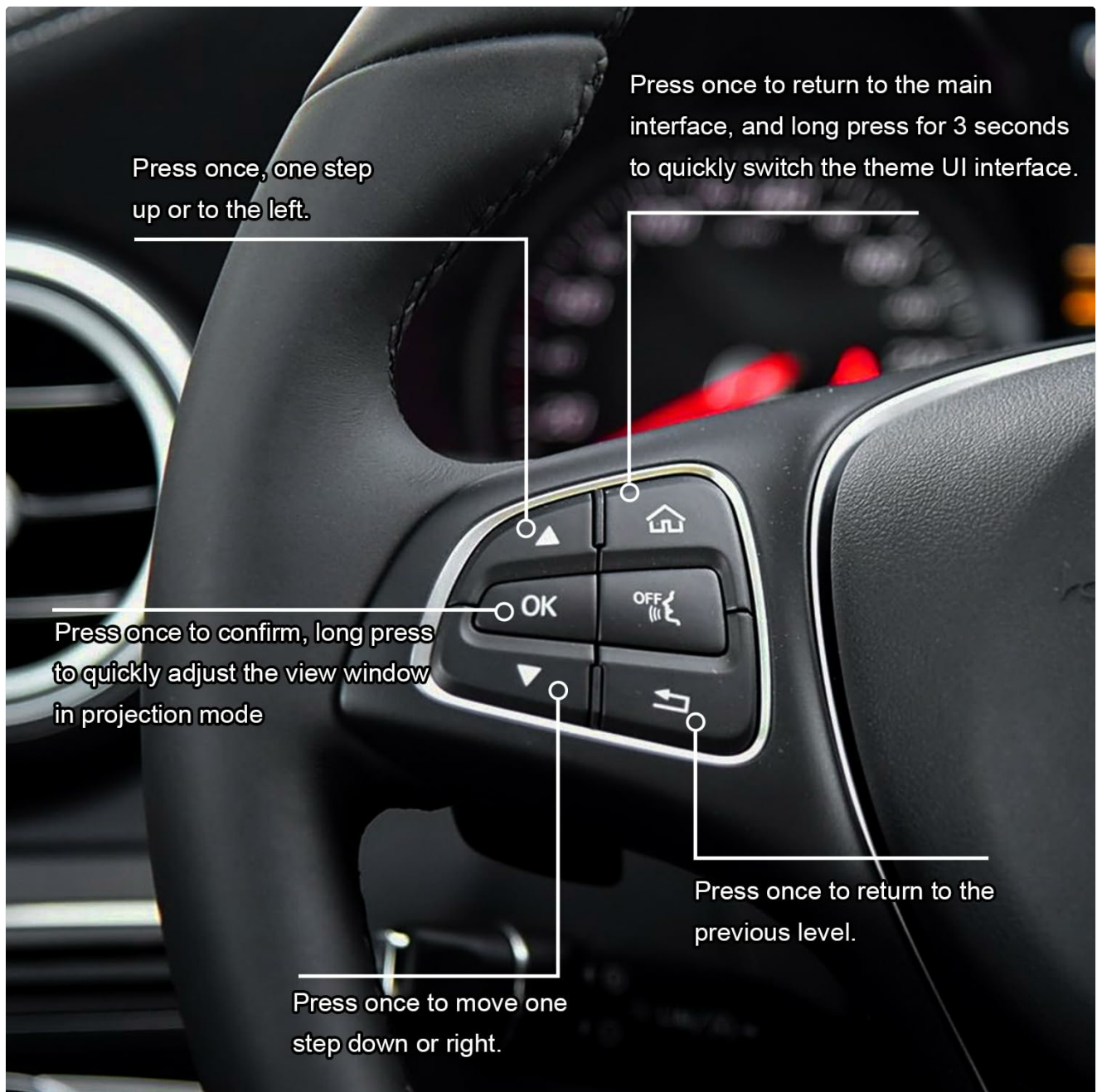
Image 5.1: Diagram illustrating the functions of steering wheel controls for the digital cluster.
