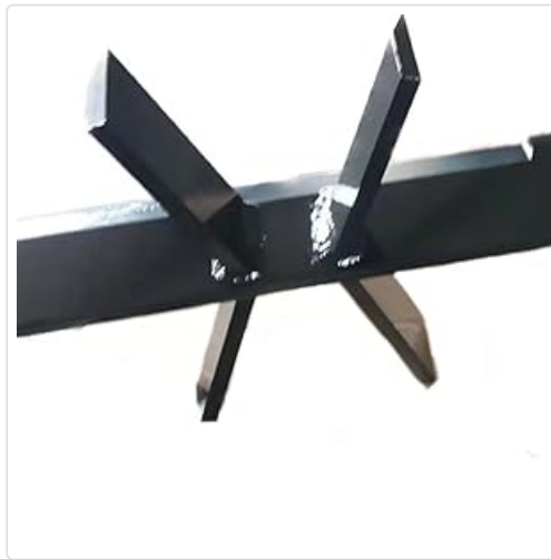
Figure 3.4: A 6-way splitting wedge, capable of dividing logs into six pieces for increased efficiency.
