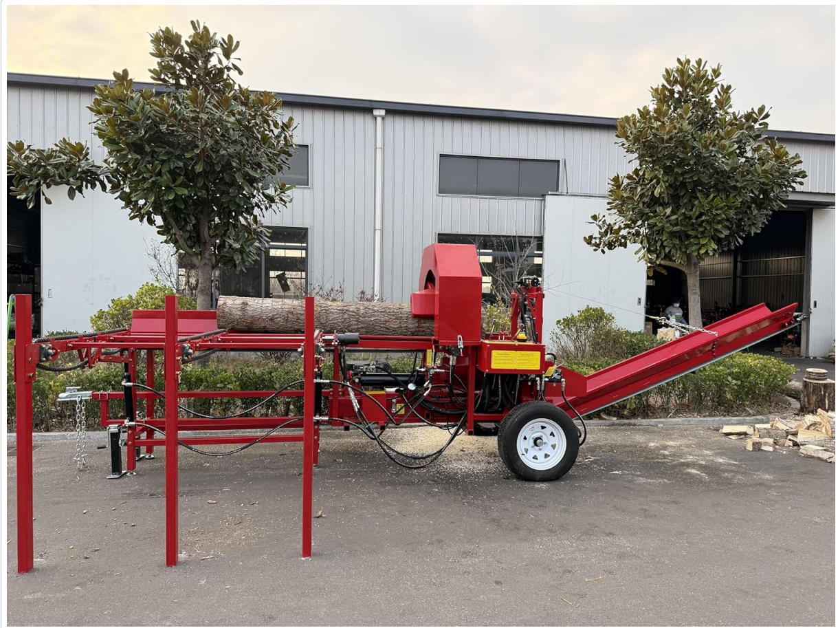
Figure 6.3: The firewood processor actively cutting a log on the feeding table, demonstrating the initial stage of wood processing.
