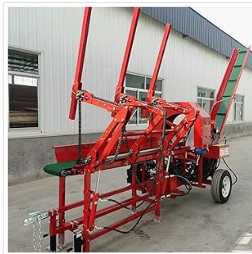
Figure 5.1: The firewood processor with its log chain table in a raised position, ready for log loading.
