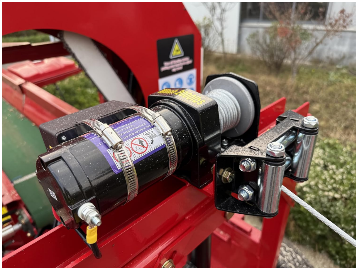
Figure 6.6: The integrated winch system, used for pulling logs onto the feeding table.
