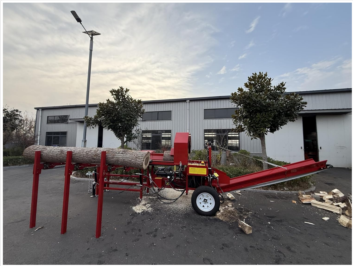
Figure 6.5: A log positioned on the feeding table of the firewood processor, ready for cutting and splitting.
