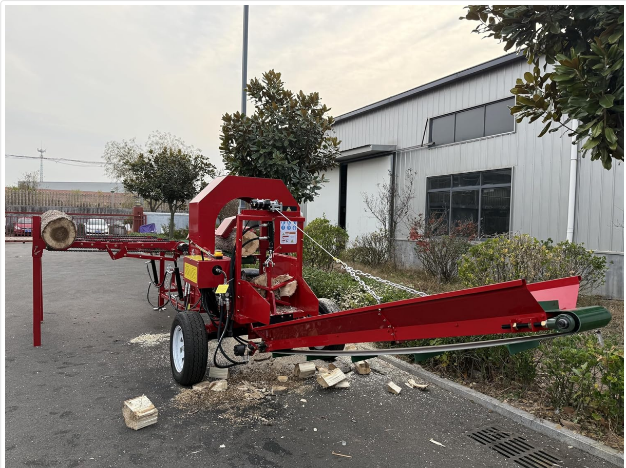
Figure 6.3: The firewood processor actively cutting a log on the feeding table, demonstrating the initial stage of wood processing.
