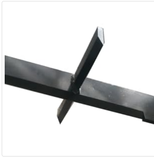
Figure 3.3: A 4-way splitting wedge, designed to divide logs into four pieces simultaneously.
