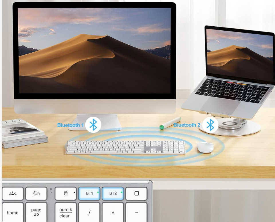
Image 3.3: The keyboard connected to an iMac via Bluetooth 1 and a MacBook via Bluetooth 2, illustrating multi-device connectivity.
