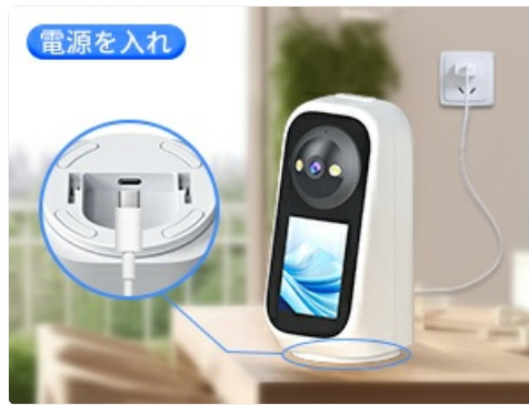
Figure 2.1: Connecting the power cable.
