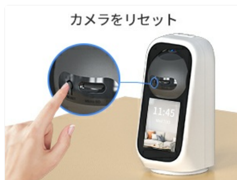
Figure 2.3: Pressing the camera reset button.
