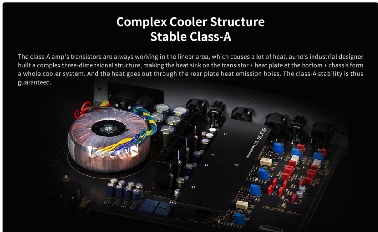
Figure 9: Internal view of the 3-dimensional cooler structure
