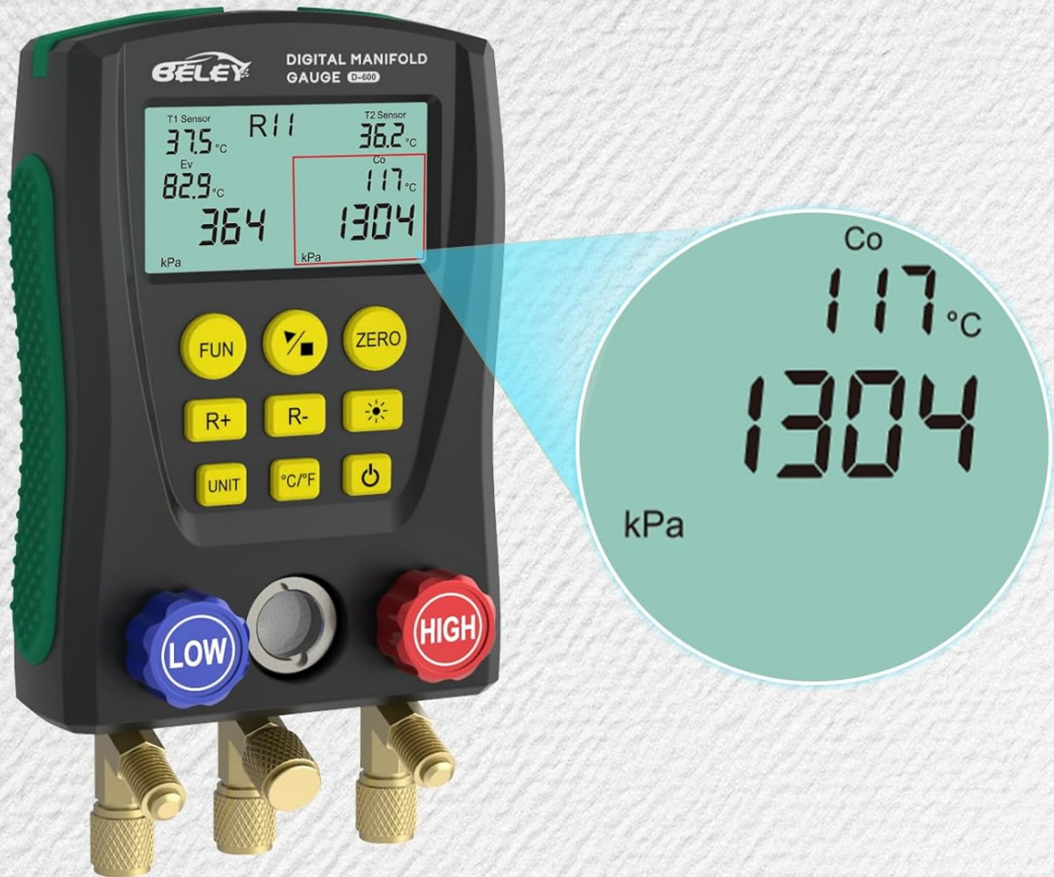
Figure 6: Condensing Pressure & Temperature Test.
