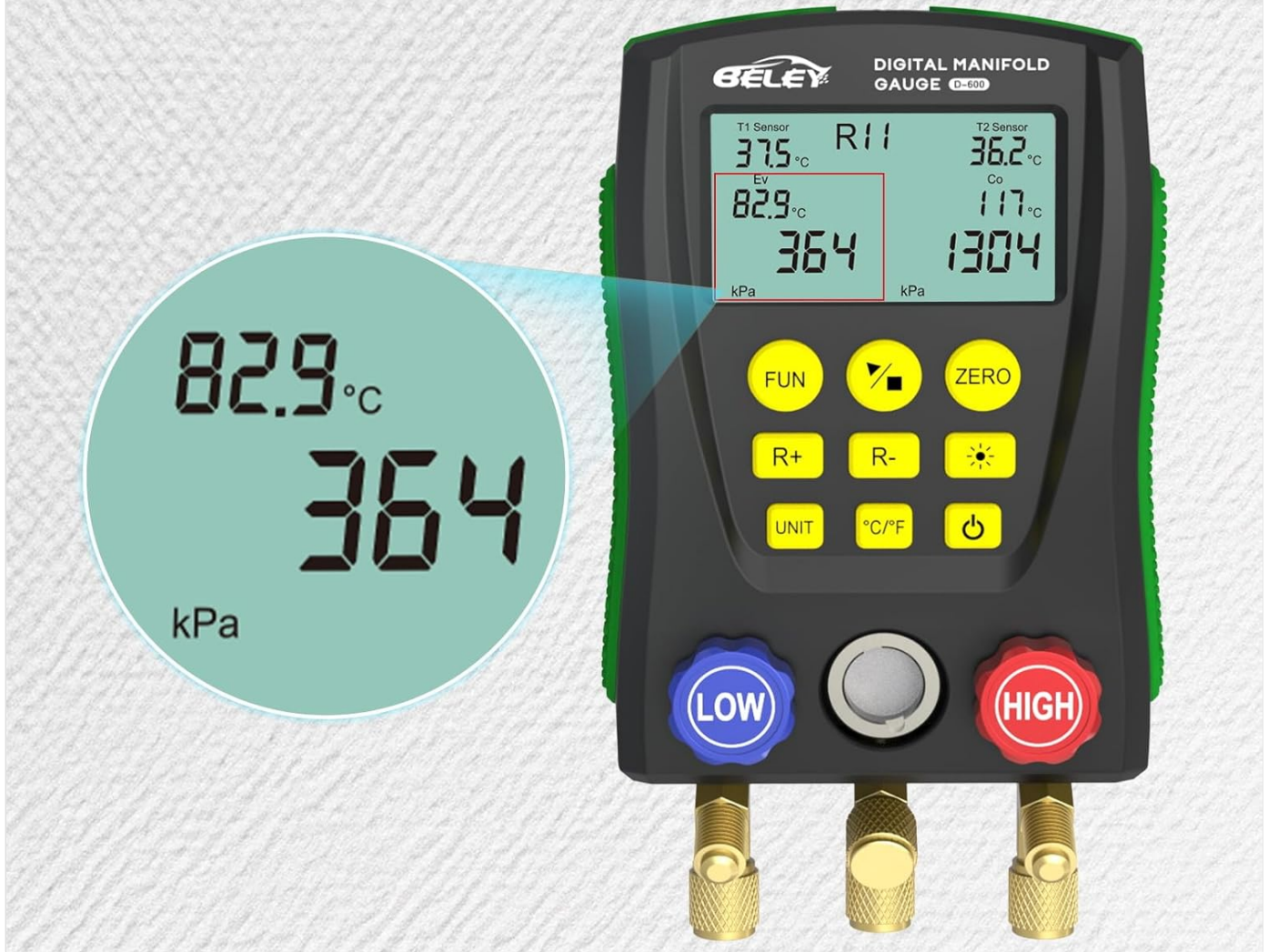
Figure 5: Evaporation Pressure & Temperature Test.
