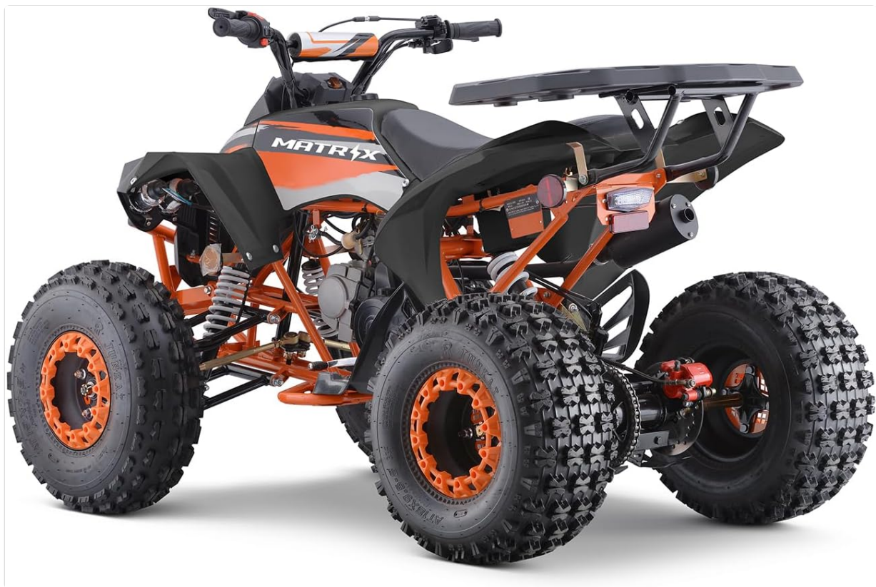
Figure 4: Rear view of the ATV. This image shows the chain drive and rear hydraulic disc brake, key components for maintenance checks.
