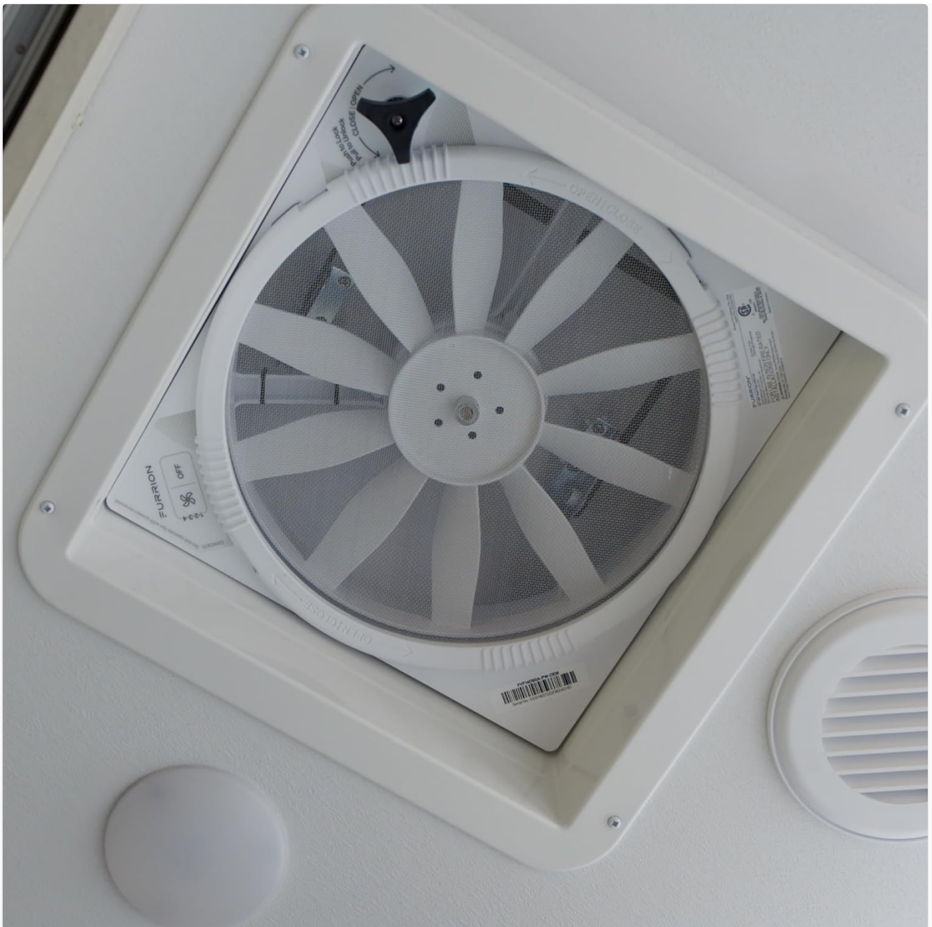
Image: The Furrion RV vent fan installed flush with an RV ceiling, showing its integrated appearance and the fan blades visible through the insect screen.
