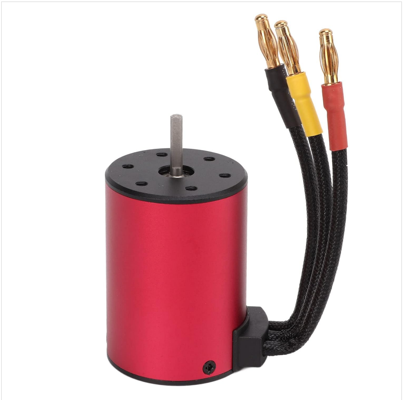
Figure 4.3: The S3650 5200KV Brushless Motor, shown here, has a diameter of approximately 36mm (1.4in) and a length of 50mm (2.0in) excluding the shaft. The shaft length is 15mm (0.6in) with a diameter of 3.175mm (0.1in). It features 4.0mm golden banana plug connectors.
