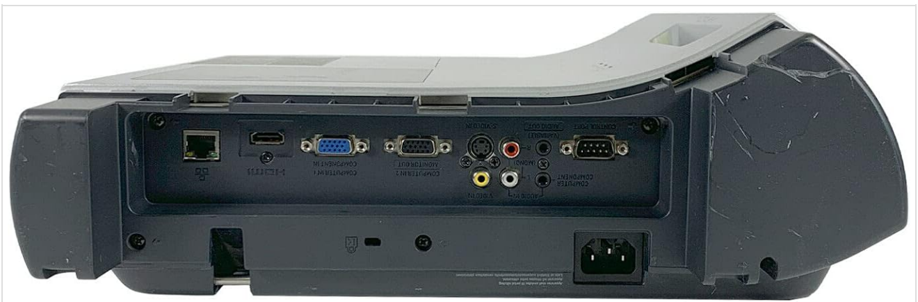
Image: Rear panel of the projector, showing various input and output ports including HDMI, VGA, Composite, LAN, and RS232.
