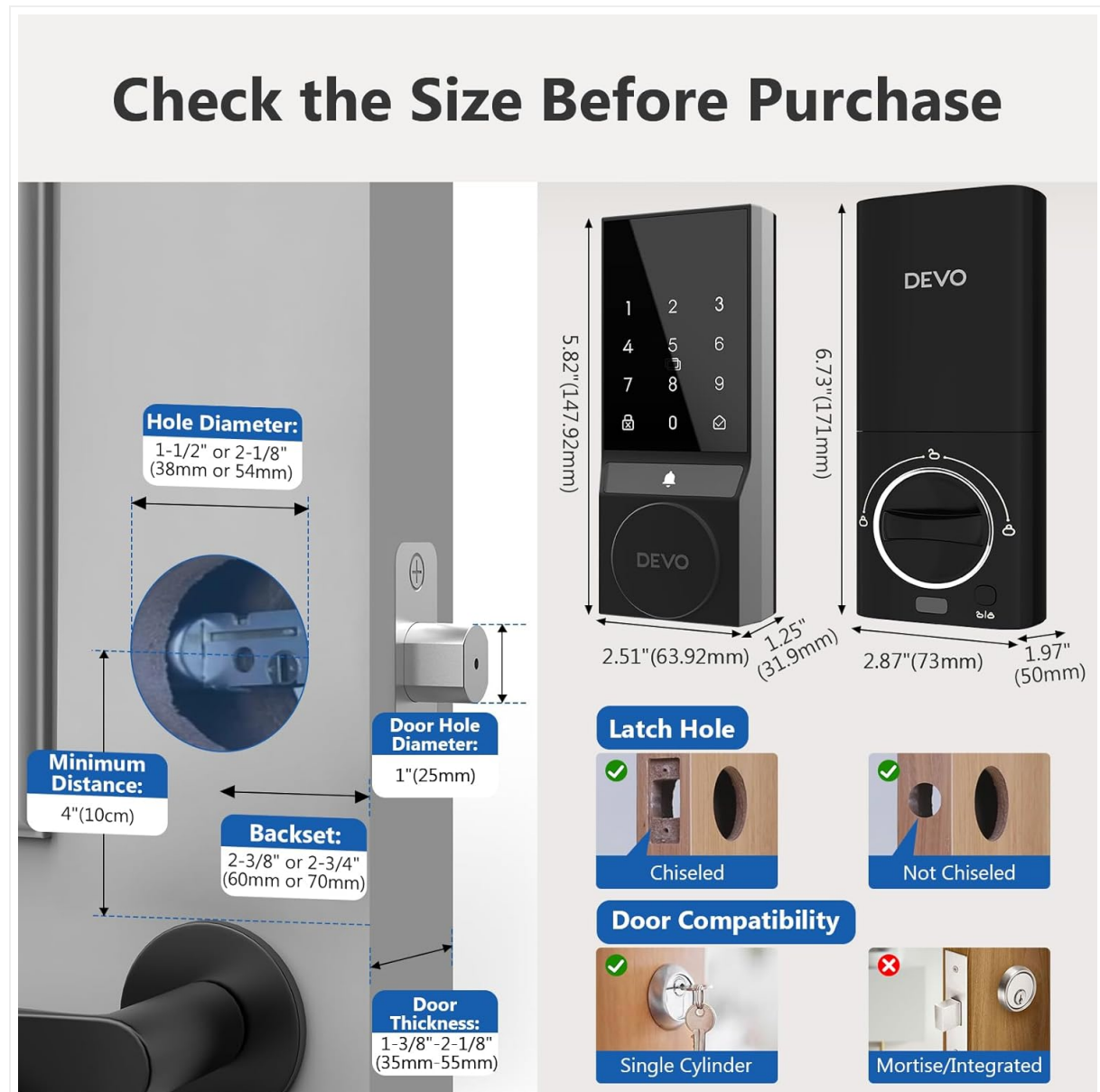
Image 3.1: Detailed diagram illustrating the required door dimensions and compatibility for installing the Devo G5 Smart Lock, including hole diameter, backset, door thickness, and latch hole types.
