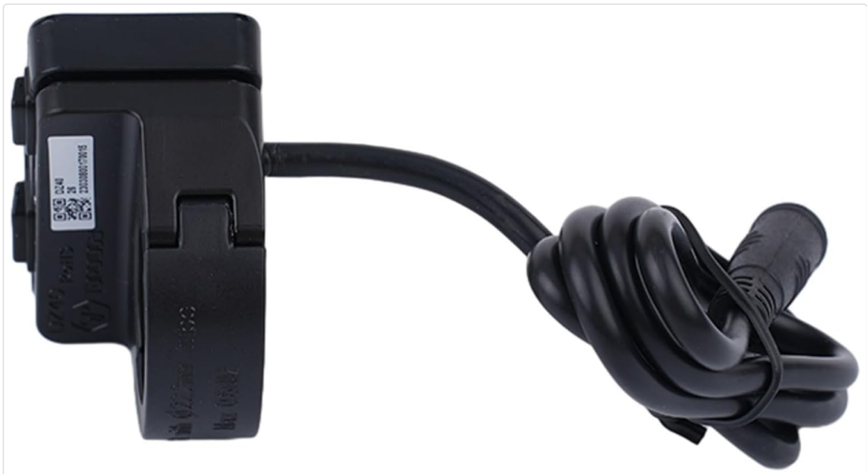
Figure 4.2: Rear view of the DZ40 display, indicating compatibility with Ø22.2mm tubes and showing a QR code with identifier 23030800170015 .
