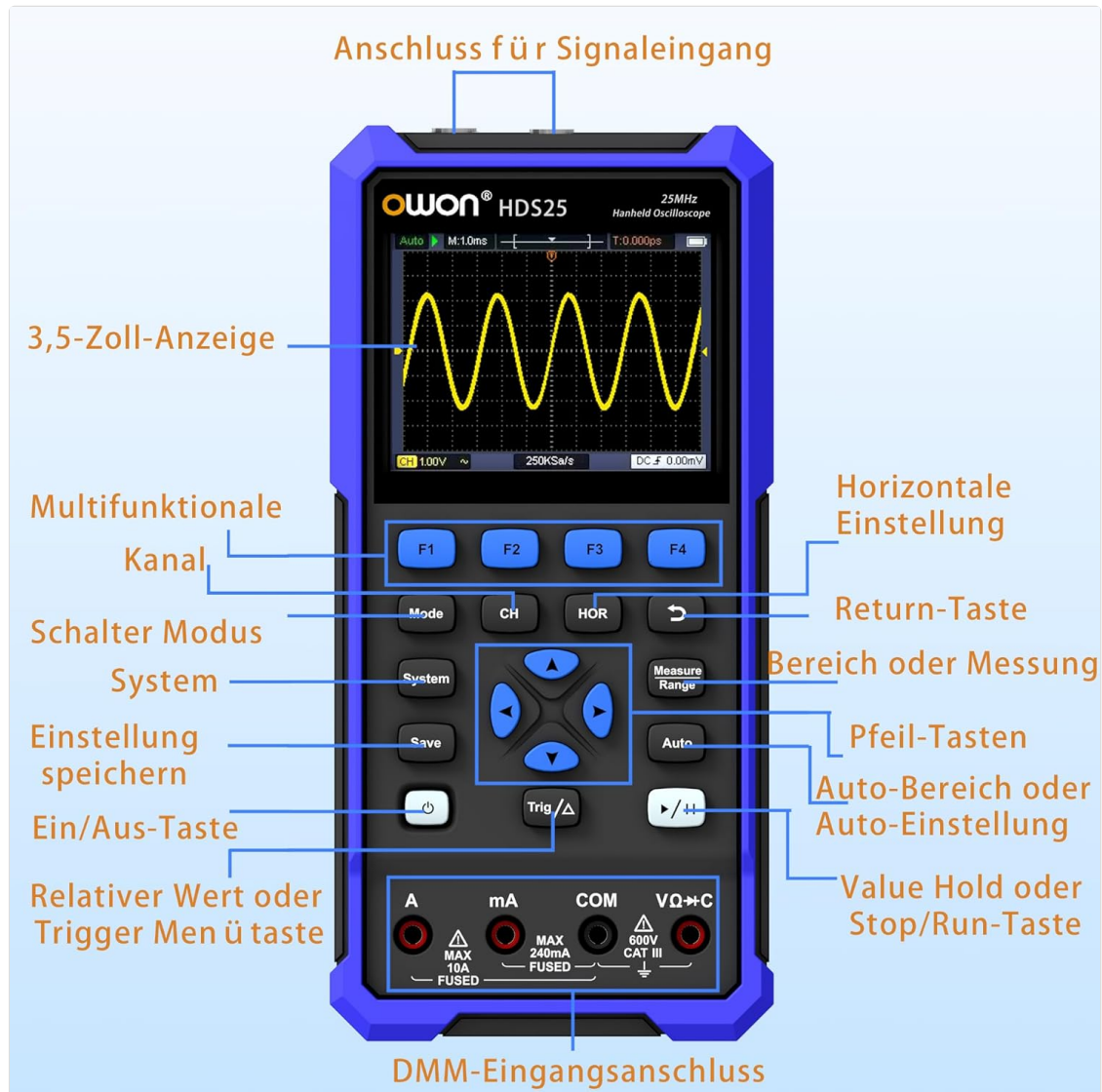
Image 4.1: Front view of the OWON HDS25 with key components labeled.
