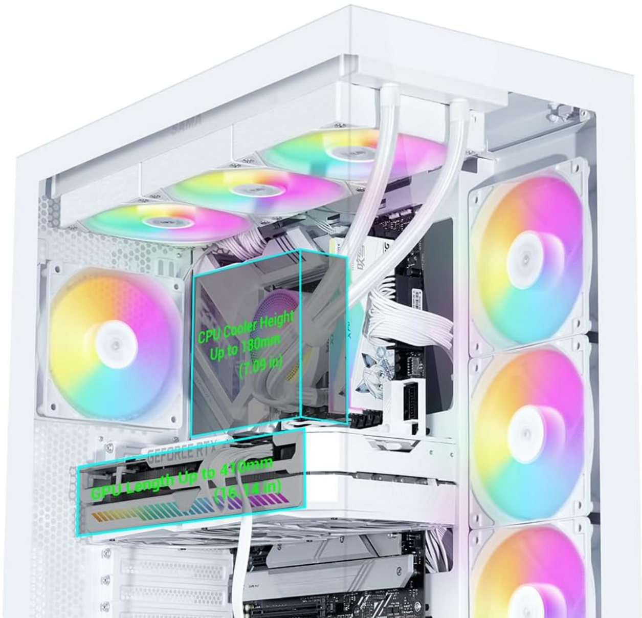
Image 5.3: Clearance for CPU cooler and GPU length.
