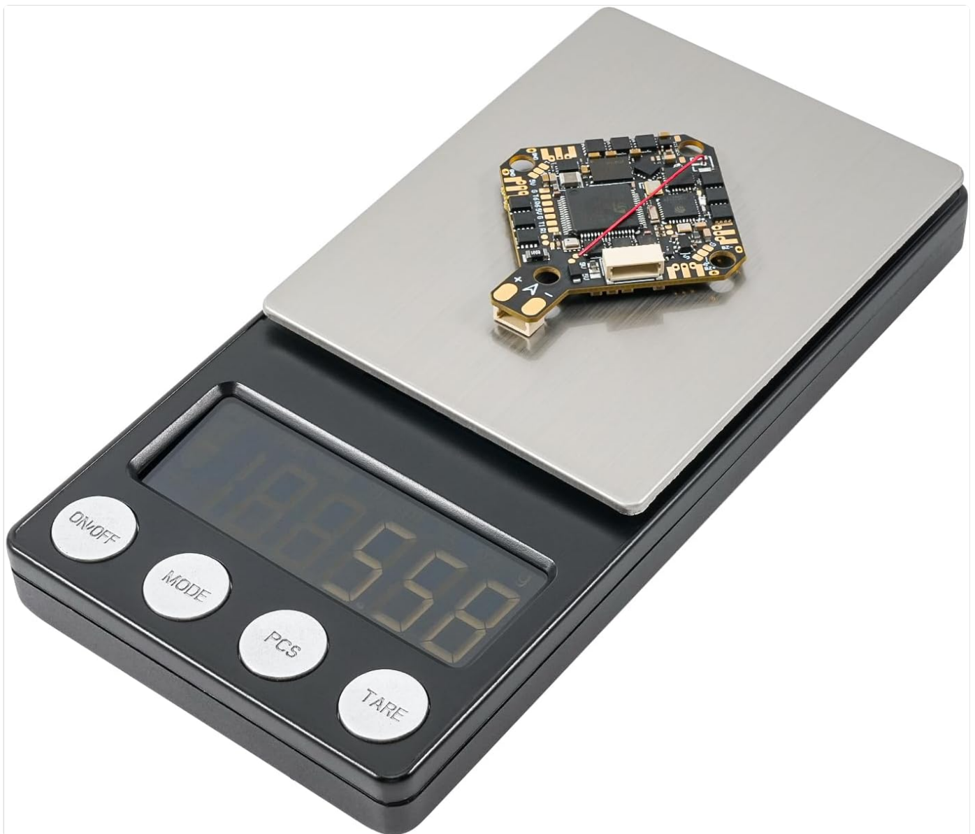
Figure 3.3: The flight controller on a digital scale, indicating its lightweight design at 5.58 grams.
