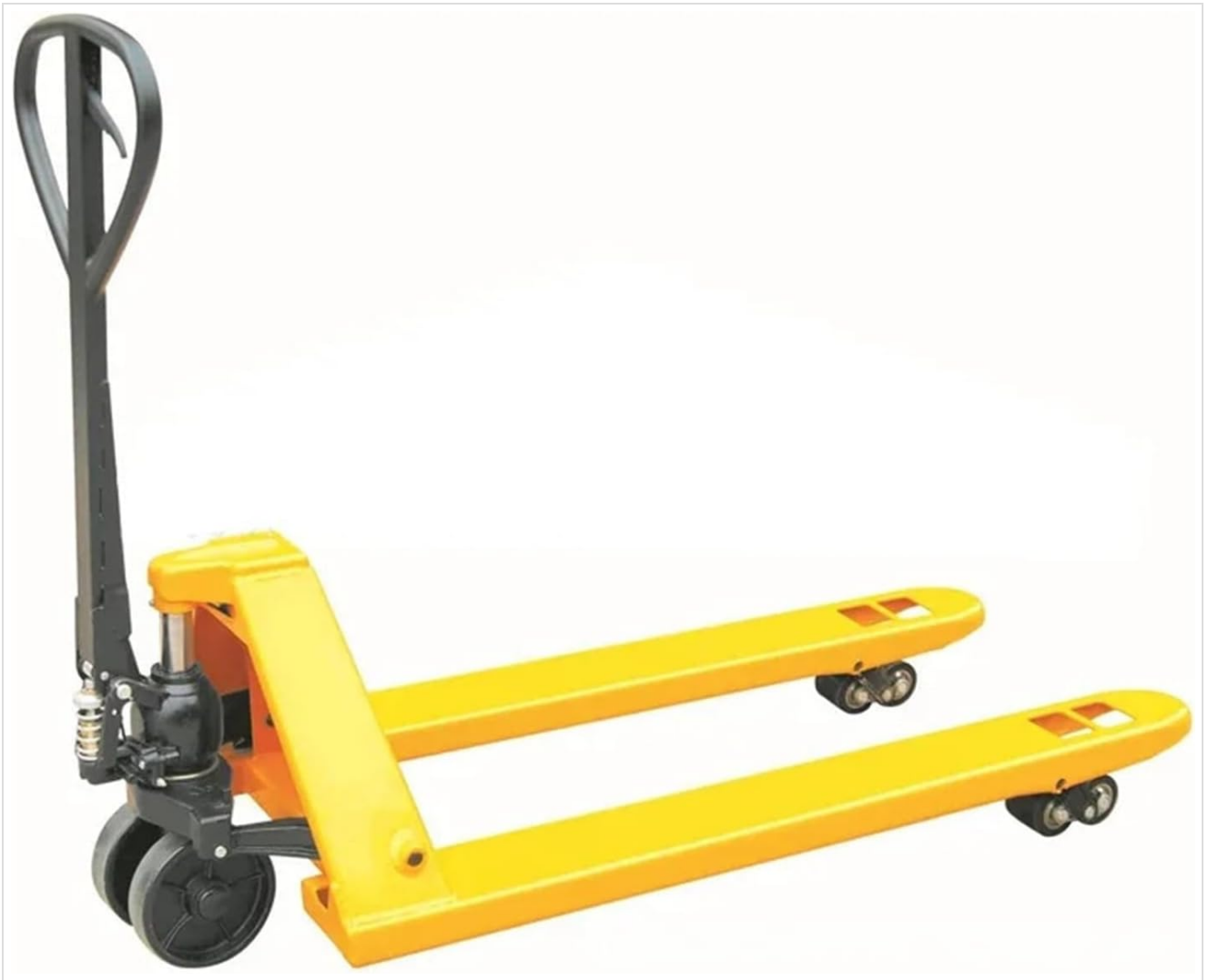
Figure 4.2: Angled view of the pallet truck from the front, illustrating the fork design and entry rollers.
