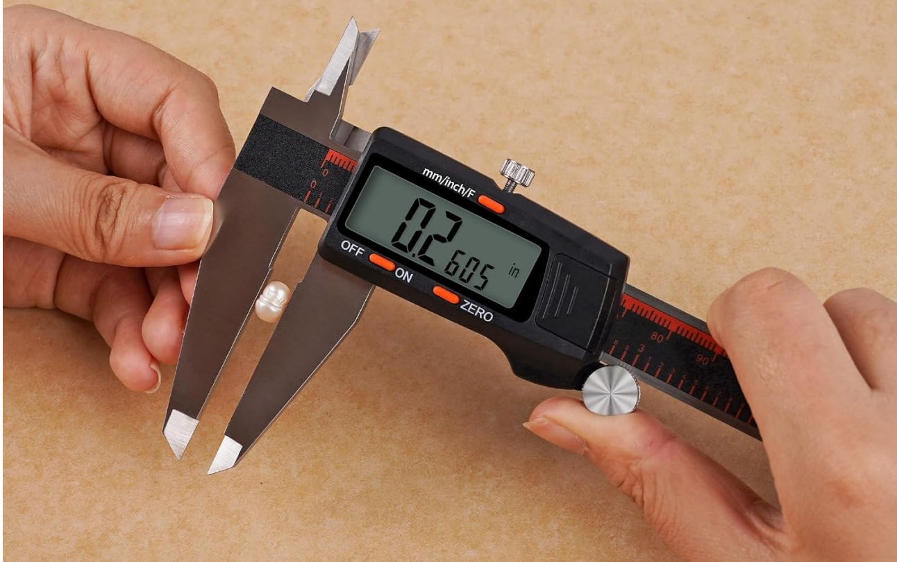
Image: Demonstrating the unit conversion feature on the caliper's display.
