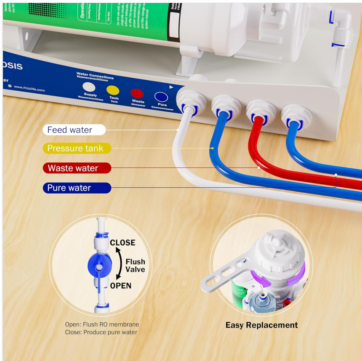
Figure 4: Water Connections and Flush Valve. This image highlights the color-coded water connection ports (Supply, Tank, Waste, Pure), the operation of the flush valve (Open for flushing, Close for pure water production), and the 'Easy Replacement' feature for filter cartridges.
