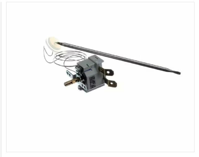
**Figure 1:** Bunn 4623-GTLU0087 Thermostat Kit. This image displays the complete thermostat kit, including the main control unit with electrical terminals, the temperature sensing bulb, and the capillary tube. The bulb is typically inserted into the liquid or air path to monitor temperature, and the capillary tube connects it to the control unit, which then activates or deactivates the heating element based on the set temperature.
